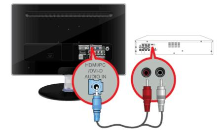
2. Connect the red and white plugs of an RCA to stereo (for PC) cable to the same colored audio output terminals of the digital output device, and connect the opposite plug to the [HDMI/PC/DVI-D AUDIO IN] terminal of the product. Press the [SOURCE] button at the front of the monitor or on the remote control to select <HDMI> mode.
